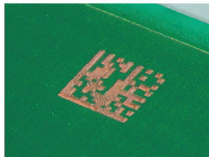
A 2-dimensional code on a printed wiring board
